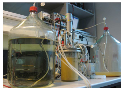
Figure 4: Continuous culture of Cryptecodinium cohnii was performed in a 3L controllable bioreactor.
